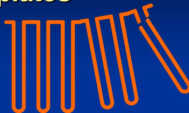
3. Etch away AAO to release ALD nanotubes
